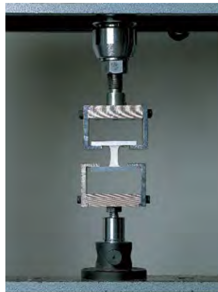
■ H-Piece Testing Jig
