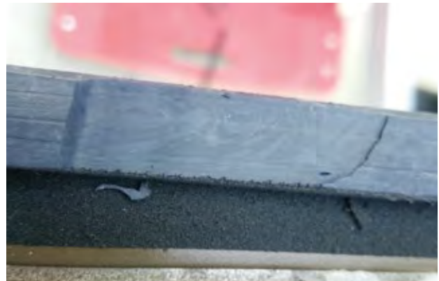
NG Mode (Insufficient mixing)
