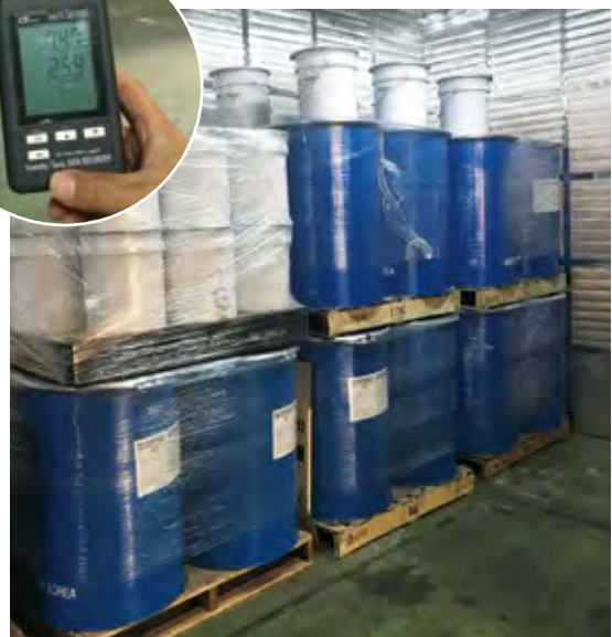
Sealants and primers must be stored under a controlled condition.
