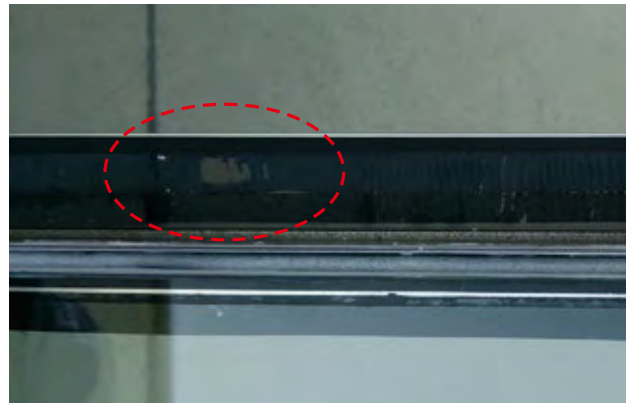
NG Mode (Adhesive failure)
