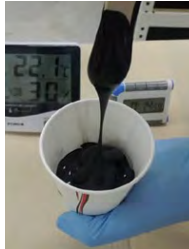
Uncured (The sealant doesn't reach snap time)
