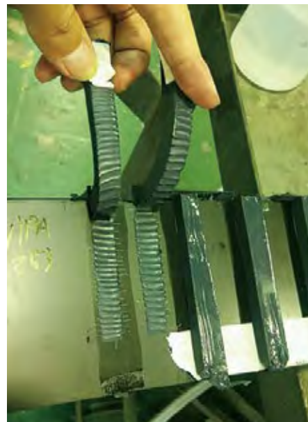
OK Mode (Cohesive failure)
