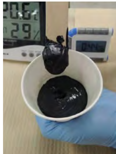
Uncured (The sealant reached snap time)
