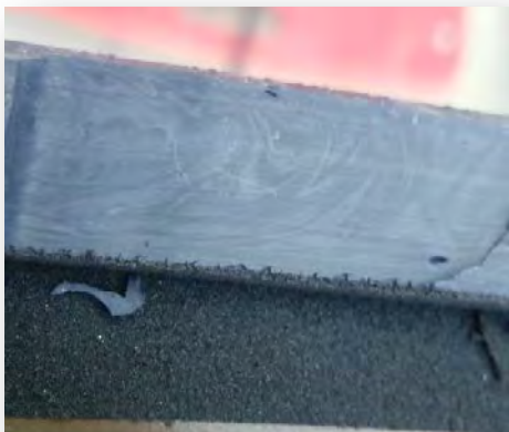
NG MODE (Insufficient mixing)
